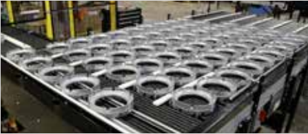
1. MULTI-LANE ACCUMULATION Accepts build-up of product flow from upstream equipment, allowing production to continue if downstream packaging machines fail.
