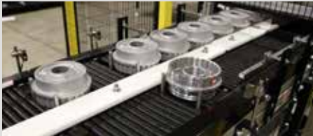
5. TRAFFIC CONTROL Using pin stops, blade stops, or brakes, release products at pre-determined intervals based on upstream and/or downstream traffic conditions and prevent jamming or overloading products during a production process.
