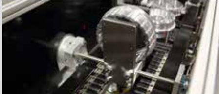
4. FLIPPER Designed to flip product 180-degrees to convey product to next stage in manufacturing process.
