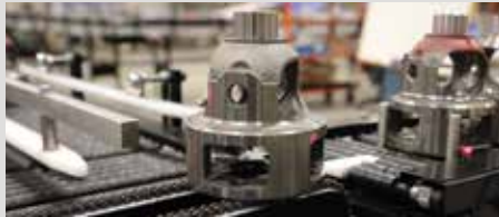
2. LIFT AND TRANSFER Lifts the product above conveyor surface and transports it 90-degrees in either direction to a predetermined point.
