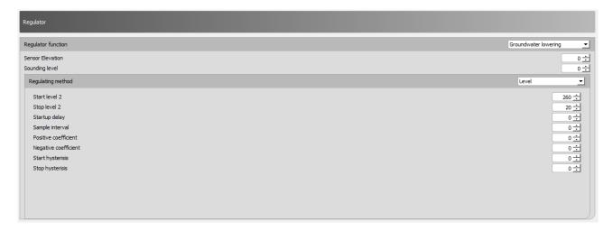
By choosing ground water level the SPIDER can keep a constant water table level. Sensor elevation is the top of the sensor tube in relation to a given terrain point. In Denmark it is called Kote DVR90. The sounding level is the sensor depth under terrain. After putting in this data simple just pick the regulation type you wish to use.
