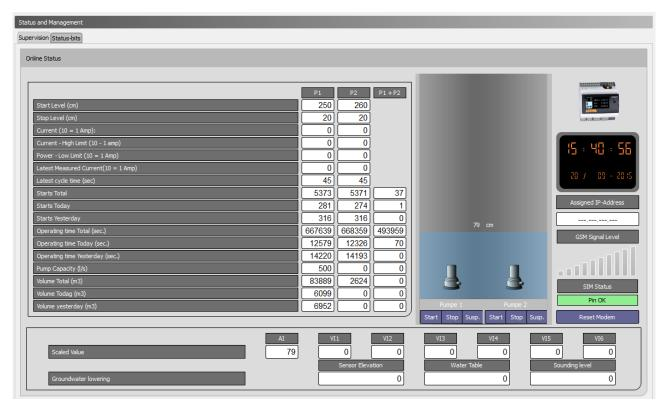
In the left frame, standard registers are displayed for the pump control, such as start/stop levels and operating parameters.
