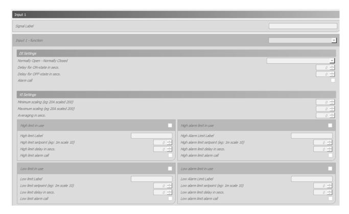
The I1-6 inputs on the SPIDER are standard 0-10 V inputs, or standard digital inputs where "0" is <5V and "1"> 12V.
