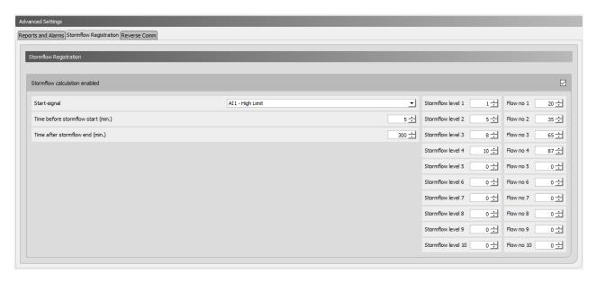
Stormflow calculation is used to record the number, duration and quantity of stormflow events.
