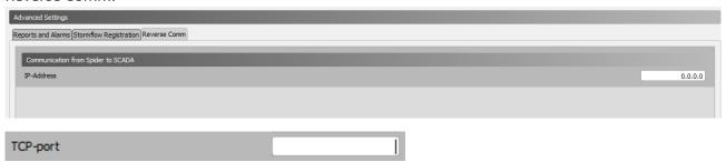
In cases where you do not have an MPLS network and you have the option of having a fixed public IP address associated with your network connection, you can make SPIDER the TCP client and then connect to the SCADA system. The IP address of the public IP address is entered along with the desired TCP port. The SPIDER will then establish a TCP connection to this address.
