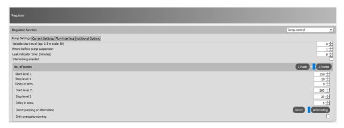
In order to use SPIDER as a pump control, select "Pump control" under the "Regulator function" setting. Here you can configure the most common parameters as shown in the picture.
