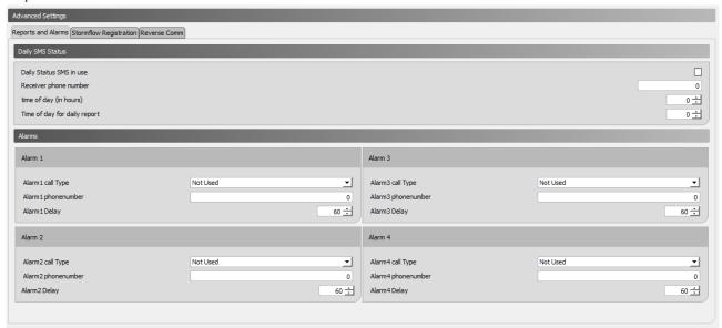
If the SPIDER is used as a stand-alone device that is not connected to a SCADA system, it is possible to receive a daily status SMS and alarm SMS in case of an alarms.
