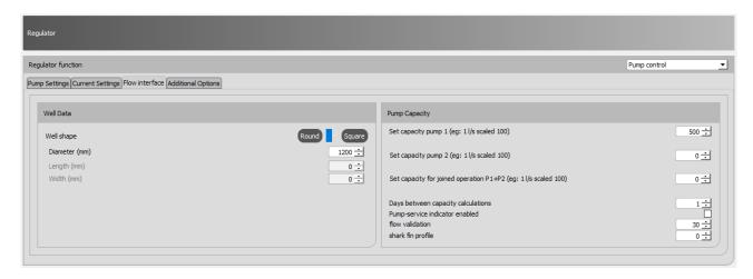
With very few settings, SPIDER can perform a validated flow calculation. You choose whether the shape of the well is round or square, then enter either diameter or the dimension of the sides in mm. This determines the surface area and SPIDER calculates based on the start/stop levels how much is pumped out during a pumping cycle.
