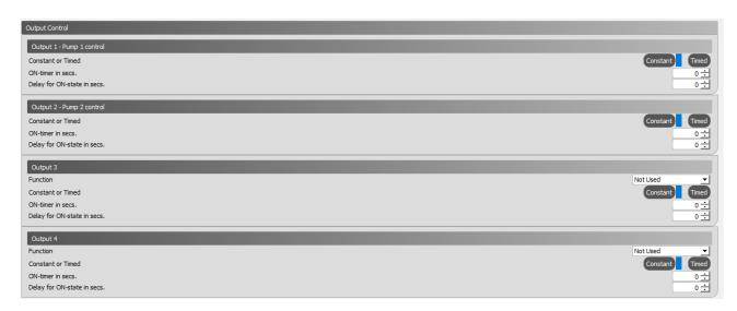
DO 1-2 are relay outputs dedicated to pump control, where DO 3-4 is used for specialized functions.
