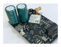
SPIDER is equipped with a built-in Power bank and can send voltage failure alarms when the primary power supply disappears.
