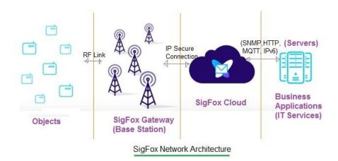
The network structure is therefore in place, which allows you to place your FIREFLY and GEKKO data loggers without having to make any further improvements. FIREFLY communicates, using already installed SigFox gateways, to the Sigfox back-end, from which data can be accessed directly via API or equivalent or via ModBus protocol through AcowaCore software.
