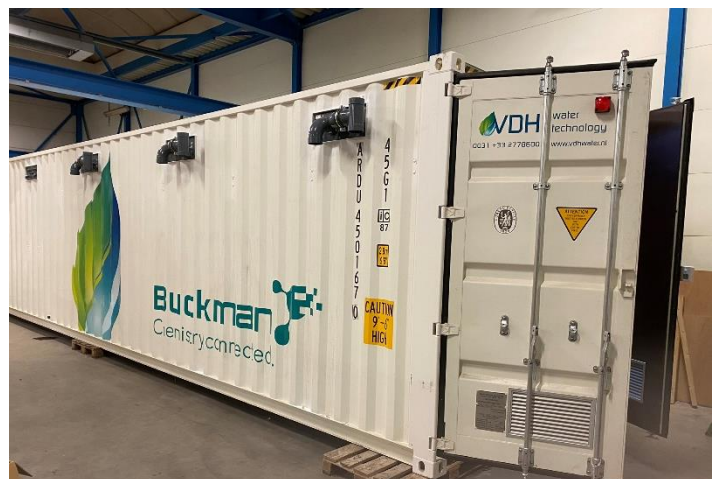
Figure 6; Mobile demonstration unit to produce low chlorate sodium hypochlorite, capacity 10 kg/h FAC.
