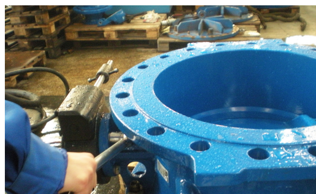
Mounting the gearbox – step 5
