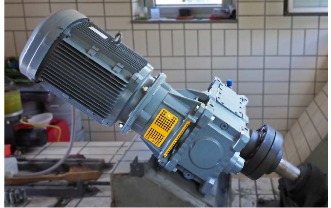
After: X series three-stage helical gear unit including energy-efficient motor, motor adapter with torsionally flexible jaw-type coupling and a pin coupling
