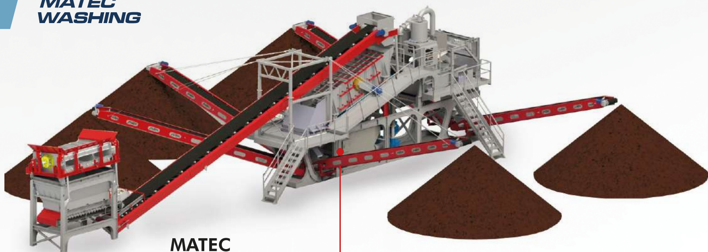
AGGRETEC SEMI-MOBILE WASHING PLANT
