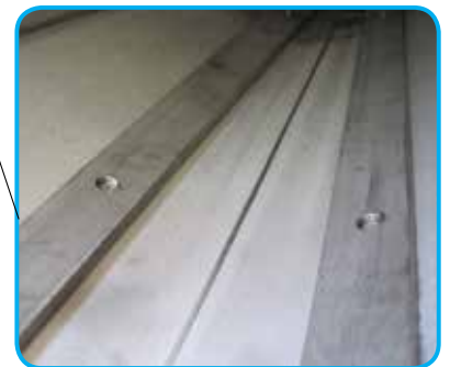
Bolted wear bars (internal view of trough)
