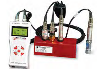
Handheld hydraulic system analyzer MC 4000
