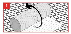
Place roll of GRIPPGrid on grishmesh floor in desired location. Roll out matting and cover length of desired area. Ensure matting is flat without kinks.
