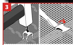
Push the clip through using a hammer. To remove clips, pry up with a flat tip screwdriver.
