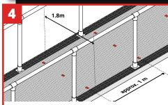
Apply clips approximately 1m/3ft apart. Use additional clips if required to ensure matting remains flat and to avoid trip hazards.
