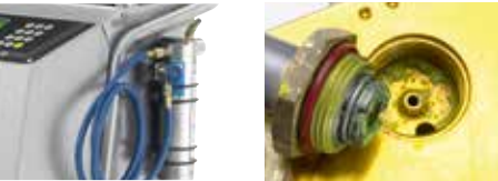
Sealant contamination in the A/C service unit without the use of the Recycle Guard
