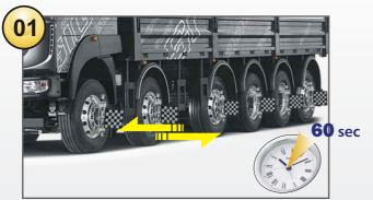
One shot Runout Compensation of 6 axles simultaneously
