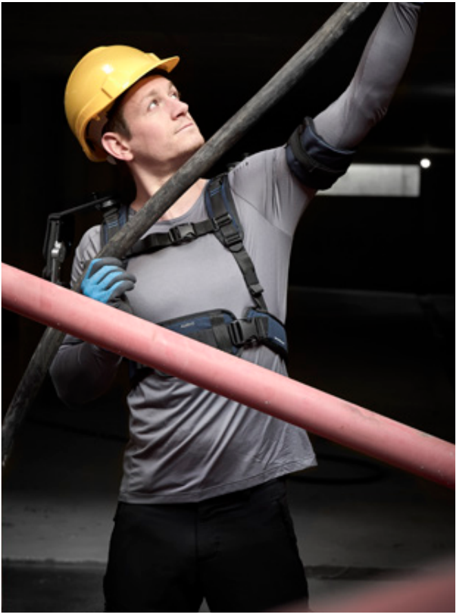
Versatility of the DeltaSuit in different fields and tasks. Scientific evaluation, show that the DeltaSuit significantly reduced muscle load and fatigue in the shoulder, neck and arms.
