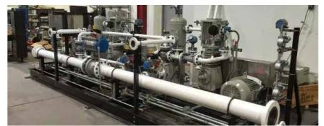
Railcar loading-offloading systems bring many benefits to a facility or project. They ensure highly accurate metering and measuring using quality pumps or compressors, filters, valves, flow meters and grounding units. These systems are often used with hazardous chemicals to ensure
