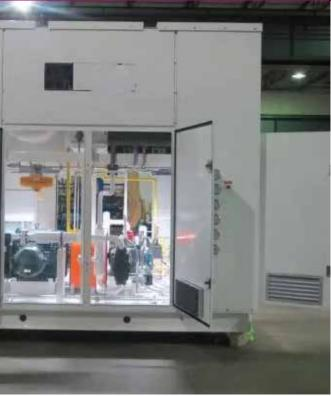
Carbis Loadtec has the design and fabrication experience to provide CNG compressor skids up to 250HP for pressure up to 350 bar. Our design and engineering team will help you select and size a suitable gas compressor to meet the demand of your specific application. Systems are designed with either electric motor or natural gas engine drivers and can include complete enclosures to protect the system from the elements and provide sound deadening where needed.
