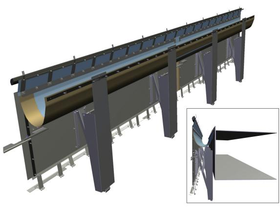
The SM1 Heavy Duty Shoe Plate Rim Seal is a liquid mounted primary shoe plate seal with a shoe mounted secondary seal. This robust seal is specially designed for arctic heavy snow load conditions. The scissor mechanism is designed and tested for a snow load of 10KN/m<sup>2</sup>.
