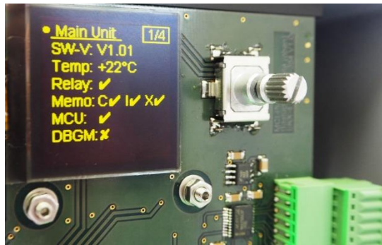
OLED Display and rotary switch for operating the menu (inside the main enclosure)
