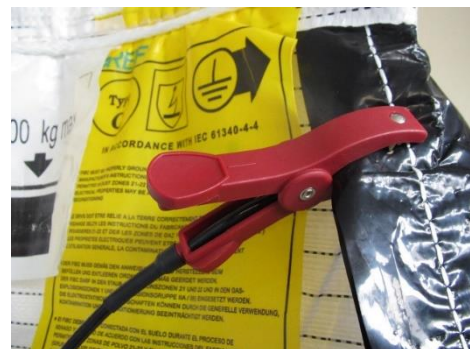
Grounding clamp on the FIBC carbon grounding tab
