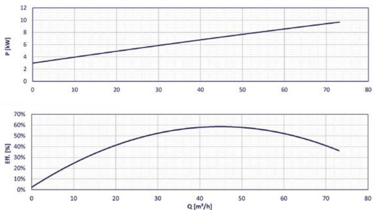
The curves and performance values refer to pumps with free delivery outlet with water at 20 °C, and two poles motor 50 Hz.
