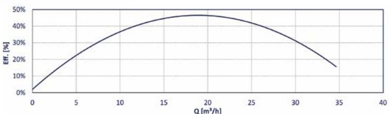
The curves and performance values refer to pumps with free delivery outlet with water at 20 °C, and two poles motor 50 Hz. These data may vary according to the construction materials, hydraulic conditions and the length of the pump.
