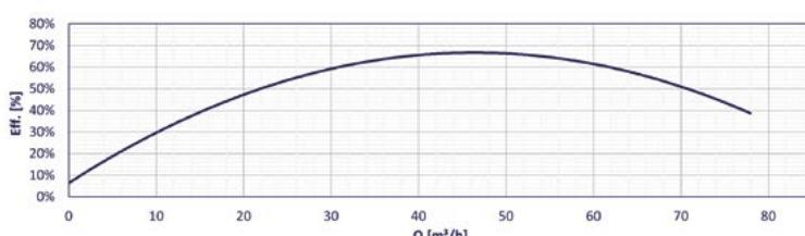
The curves and performance values refer to pumps with free delivery outlet with water at 20 °C, and two poles motor 50 Hz.
