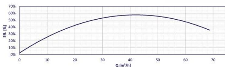
The curves and performance values refer to pumps with free delivery outlet with water at 20 °C, and two poles motor 50 Hz.
