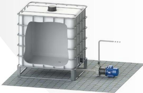
► **Installation - Positive suction:** The centrifugal pumps should only be installed with the shaft positioned horizontally in a positive suction head arrangement. Suitable devices should be fitted to prevent dry running and the formation of a vortex and possible air suction. Running dry or with air bubbles can cause damage to the mechanical seal.
