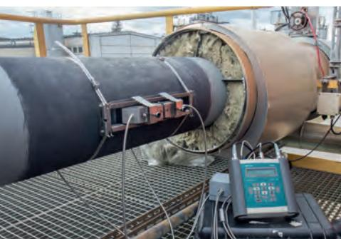
Flexim's range of FLUXUS® G60X portable gas flow meters not only covers virtually any gaseous medium, they also include all liquid flow metering capabilities of the FLUXUS® F60X series meter series making them a truly comprehensive tool.
