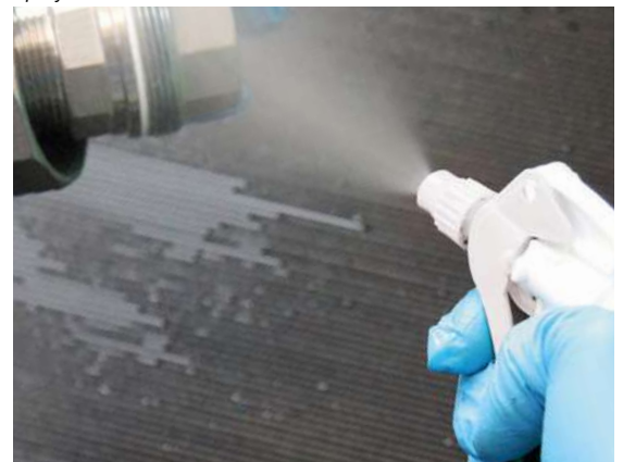
Spray on GS 200 – remove sealant
