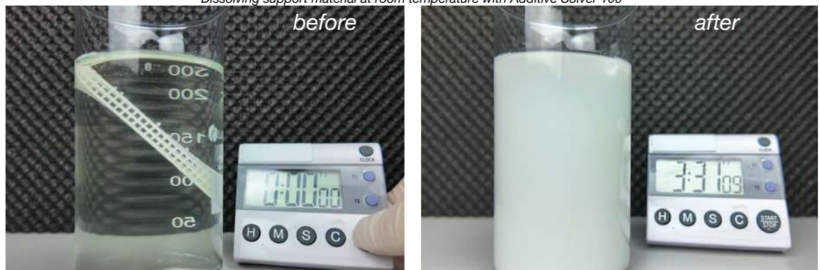
Dissolving support material at room temperature with Additive Solver 100
