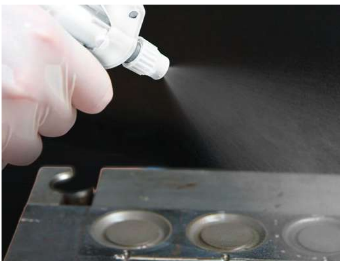
Manual cleaning of a plastic injection mould
