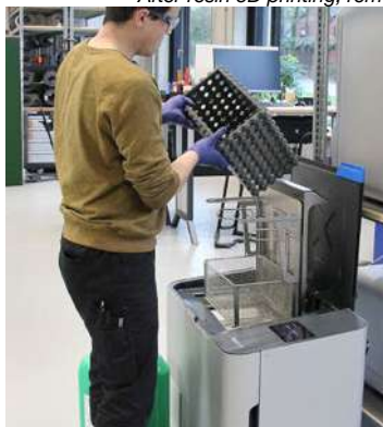
After resin 3D printing, remove uncured resins in the washing station.
