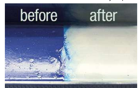
Paint removal with Poly Strip 100
