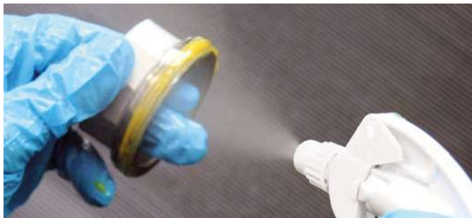
Removing sealant with GS 200
