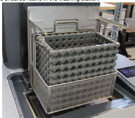
After resin 3D printing, remove uncured resins in the washing station.
