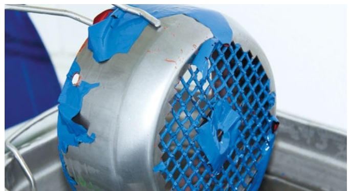
With PROLAQ L US paint removal in an ultrasonic bath
