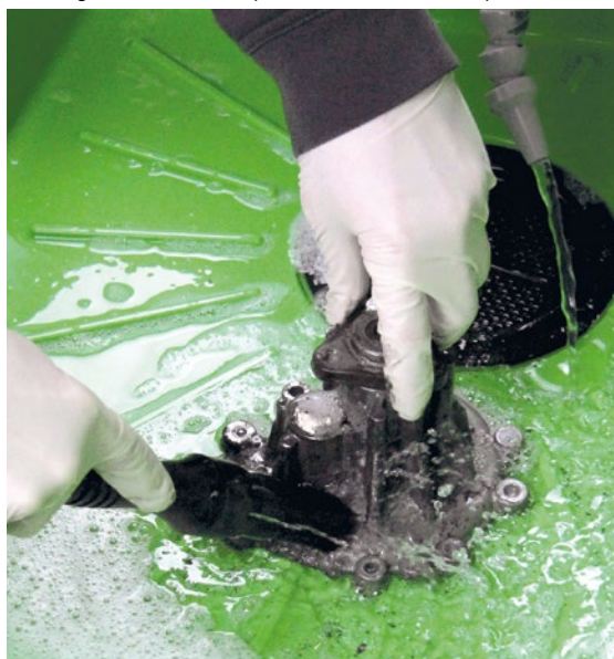
Cleaning oil-contaminated parts in the BIO-CIRCLE parts washer
