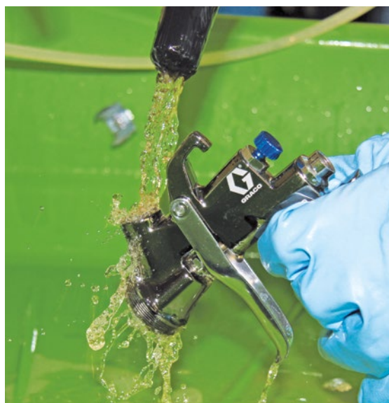
Manual cleaning of a spray gun in the PROLAQ Compact
