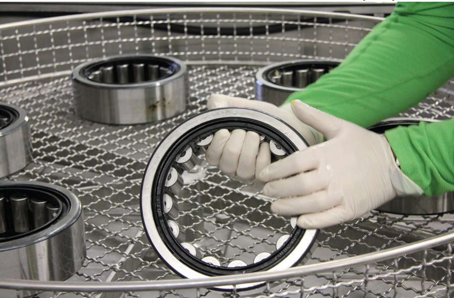
Cleaning ball bearings in the HTW
