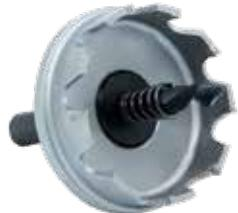
Hole cutter for hand and column drilling machines, high-quality industrial design with carbide cutting plates for high cutting performance, with centre drill (exchangeable) and ejector spring
