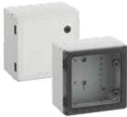
Cabinet - Industrial Quality, suitable for installation in harsh environments and in exposed outside areas, box and frame: glass-fibre reinforced polycarbonate, grey, similar to RAL 7035, door: Polycarbonate. Door latch: sash fastener with 3mm double-bit insert (interchangeable) in accordance to DIN 43668
