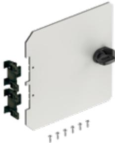
Inner door made of insulating material for installation in GEOS cabinets, incl. fixing material and rotary twist lock, 3mm double bit, for individual use, e.g. for installation of displays, command and signalling devices, material thickness: 4 mm
