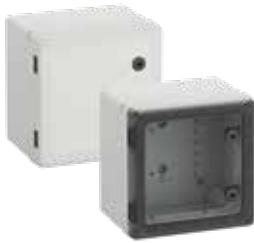
Cabinet - Industrial Quality, suitable for installation in harsh environments and in exposed outside areas, box and frame: glass-fibre reinforced polycarbonate, grey, similar to RAL 7035, door: Polycarbonate.
