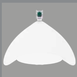
FLATWIDE symmetric wide beam beam angle: approx. 90 degrees
