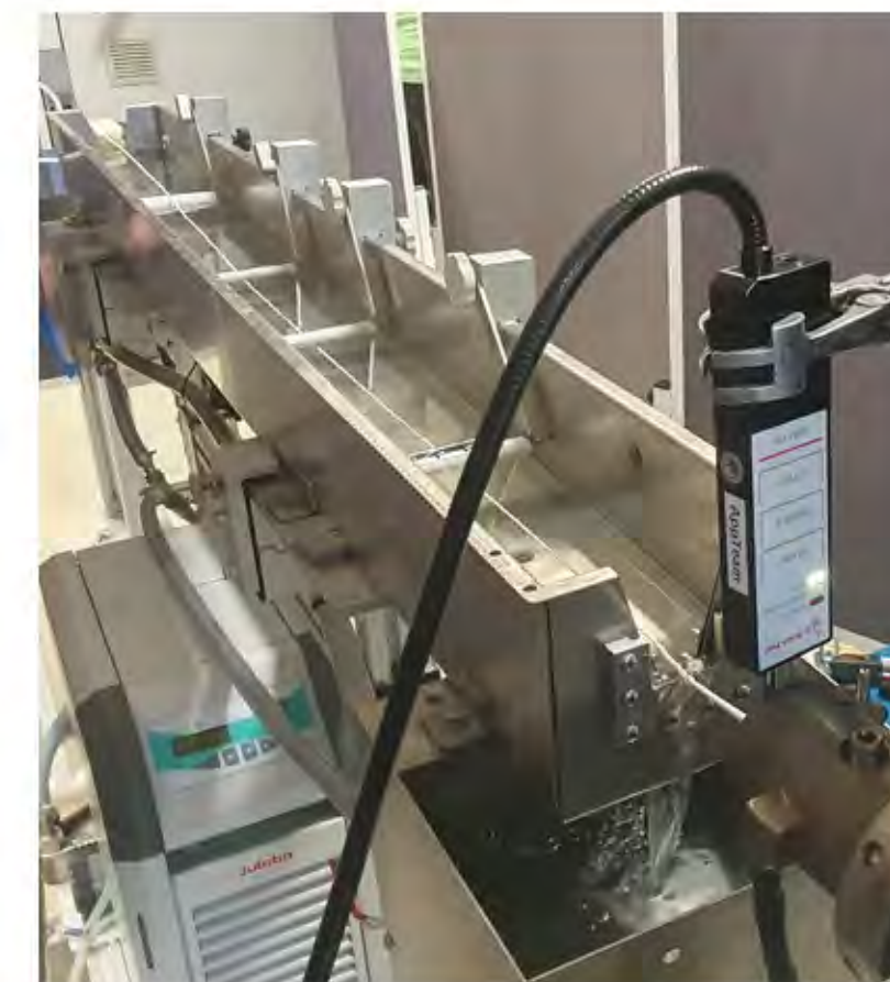
Figure 24: Experimental setup with the Raman probe directly outside of the die head with the polymer strand being cooled in a water bath and pelletized.
