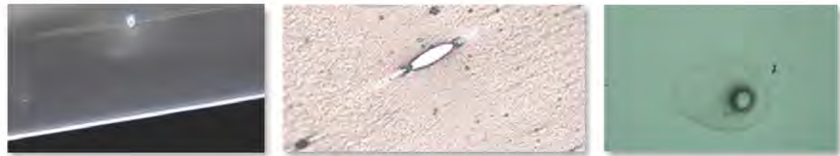
Figure 32: Exemplary defects in a plastic film according to ASTM D7310 – 21.
