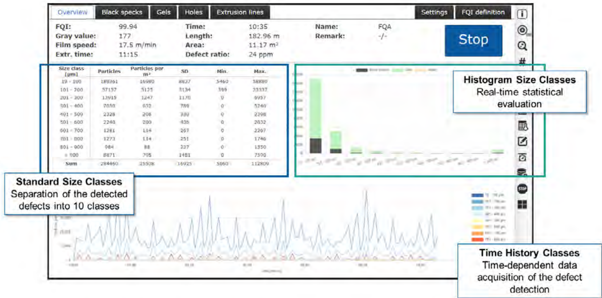
Figure 34: Statistical evaluation of film quality analysis and classification of defects.
