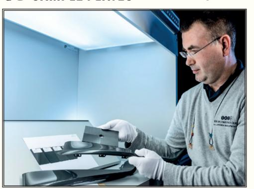
The color is assessed both visually and using state-of-the-art measurement technologies including a Konica Minolta spectrophotometer. If the customer wishes, we are happy to evaluate the results with them in conjunction with our COLOR COMPETENCE CENTER. This gives us the possibility of a direct exchange of views on fine tuning, with immediate modifications if necessary.
