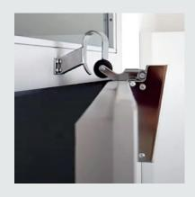
Door dampers are usually installed centered on the upper edge of the door. The hook sits above it on the door frame. When the door is opened, the hook automatically pushes the roller lever down, tensioning the built-in spring.
