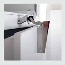
If the door is flung shut, the roller lever swings upwards when it reaches the hook, cushioning the motion of the door hydraulically in the process. The damping is progressive, which means that the doors are cushioned smoothly regardless of size and weight even if they are thrown shut very quickly.
