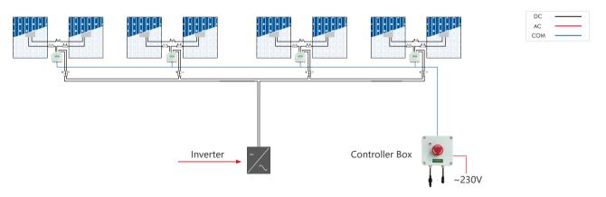
Note: The control box can convert AC 230V to DC 24V, and then control the working status of PEFS. PEFS-PL can be powered by EPS output while used in a solar storage system.
