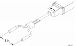
Use the Y-lead adapter to extend the reach of the probe and to connect to 0.025 inch square pins spaced as far as 1.5 inches apart. Use with Square pin adapter.
