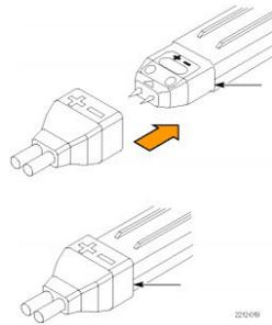
Use the square pin adapter to connect the probe to other accessories, such as the Y-lead adapter.
