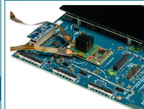
16 GHz solder down, Long-Reach, flex-circuit accessory provides a probing solution for DDR and LPDDR electrical validation when used with Nexus XH Series Interposers. The FLR tips' increased flexibility and long reach helps access inaccessible test points. Each tip has a stored factory AC calibration and a nominal XH series interposer response which is de-embedded automatically on the instrument.
