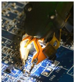
The browser tips are constructed of high strength BeCu and super-ceramic resistors. Each pin has integrated pogo springs and a crown cut tip to help make solid mechanical connections to components and traces.
