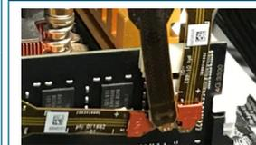
16 GHz solder down, flex-circuit accessory provides a probing solution for DDR4 and LPDDR4 electrical validation when used with Nexus XH Series Interposers. Each tip has a stored factory AC calibration and a nominal XH series interposer response which is de-embedded automatically on the instrument
