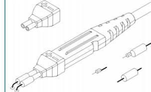
Use the solder-in adapter with the resistors and wires in the kit to create soldered test points to your circuit.
