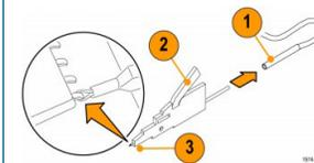
Use the IC Micro-Grabber to probe the leads on integrated circuits that are surface-mounted.
