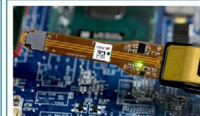
20 GHz solder down, flex-circuit accessory with an active buffer amplifier on its tip. Each tip has a stored factory AC calibration which is de-embedded automatically on the instrument
