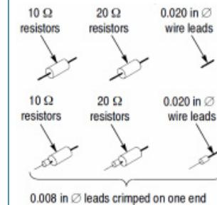
0.008 in  $\varnothing$  leads crimped on one end
