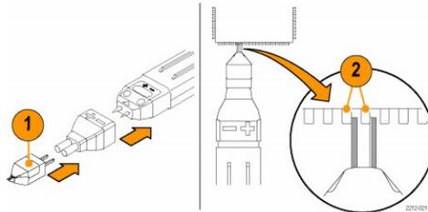
Use the TwinFoot adapter to probe two adjacent leads on a surface-mount integrated circuit. Use with Solder-in Adapter.
