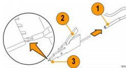
Use the IC Micro-Grabber to probe the leads on integrated circuits that are surface-mounted.
