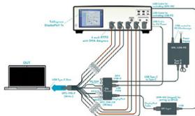
The P77C292MM adapter includes TriMode functionality enabling differential, single ended, and common mode measurements. Include variable termination voltage that can be set manually or automatically using voltage sense circuitry in the P7700 or TDP7700 probes over a range of  $\pm 4$  V for testing display technologies like HDMI and Display Port.
