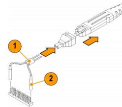
Use the Y-lead adapter to extend the reach of the probe and to connect to 0.025 inch square pins spaced as far as 1.5 inches apart. Use with Square pin adapter.
