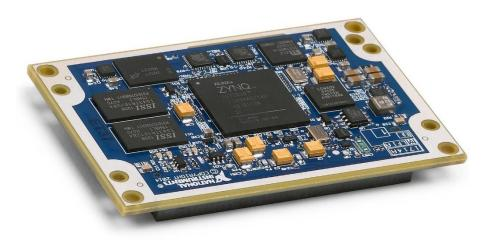
Figure 3 CompactRIO System on Module, sbRIO-9651 (SOM)
