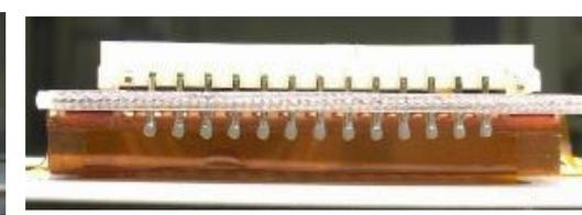
**No drooping and can be used for through-hole reflow.**
