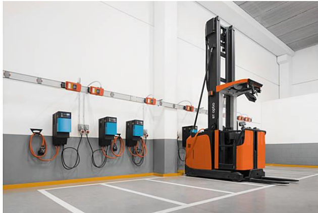
Figure 1 A forklift with Li-Ion batteries is being charged
